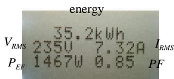
**Fig. 4.** Photograph of the energy meter LCD panel, monitoring after a few days operation.
