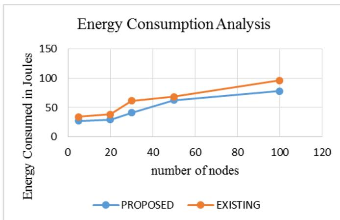
Figure 4: Energy consumption analysis for packet size 256 bytes
