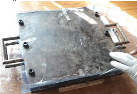
Fig no 1: preparation of laminates by hand layup method
