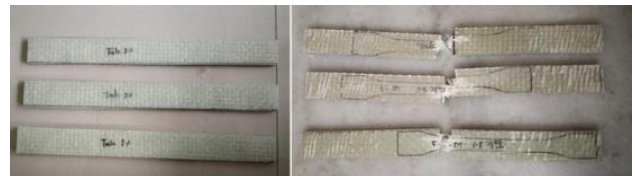
Fig no 4: Specimens before and after tensile test
