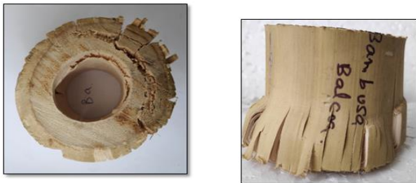
Fig.3 Failure of bamboo specimens under compression test
