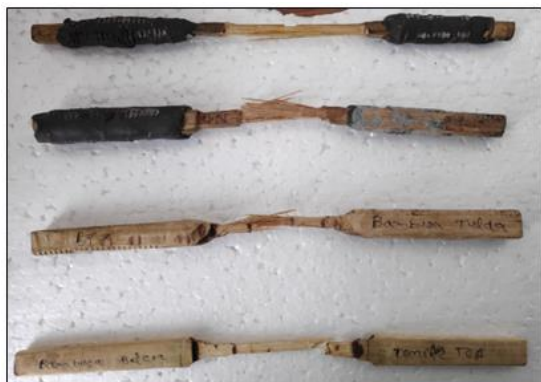
Fig.11 Failure in tensile specimen
