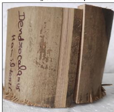
Fig.14 Failure in shear specimen
