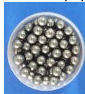
Fig.2. Container with Particle damper
