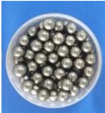
Fig. 5 Particle damper of spherical particles 9 mm
