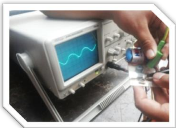
Fig. 5. Testing with Electronic Product Oscilloscopes from a Water Detector
