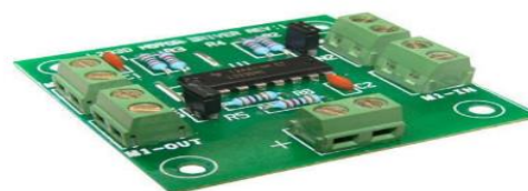
Fig 7. L293D Motor Driver
