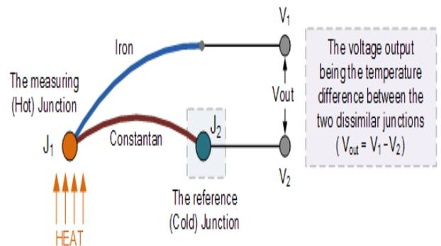
**Fig 3: Principle of Temperature Sensor**
