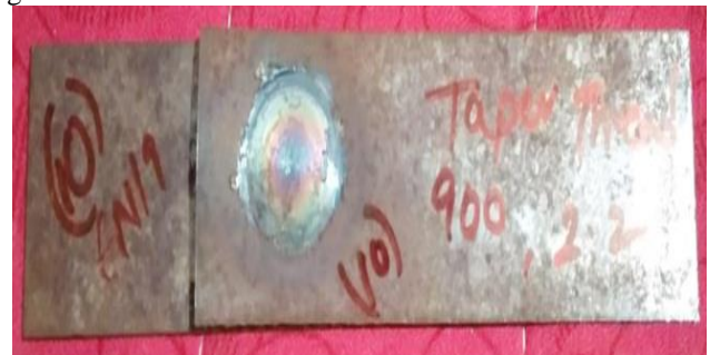
Figure 6: Al6082-Al6082 Welded Specimen
