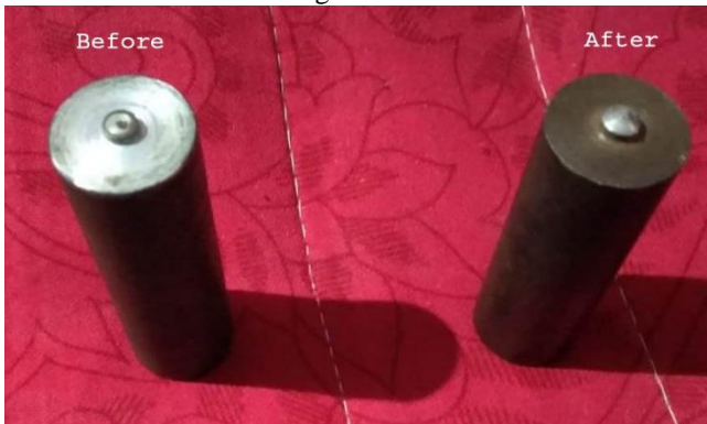
Figure 8: EN19 Tool Blunt while doing on MS Plates
