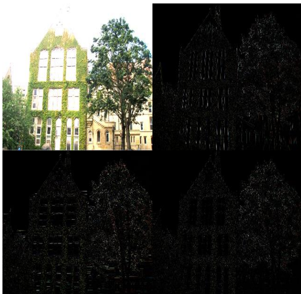
Figure 3. Compression of the image based on the Daubechies wavelet by a factor of 6.
