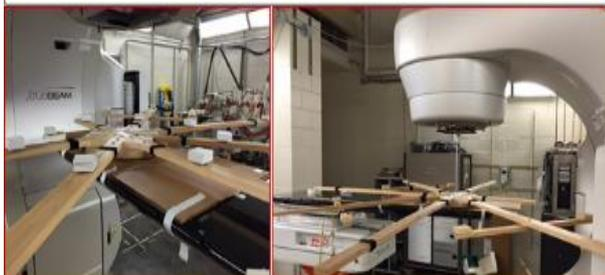
Figure .1 Measurement Locations: Out-Beam in the patient plane (23 points) and Measurement setup.
