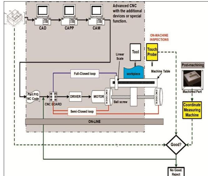
Fig. 1: Current advanced CNC system [5]
