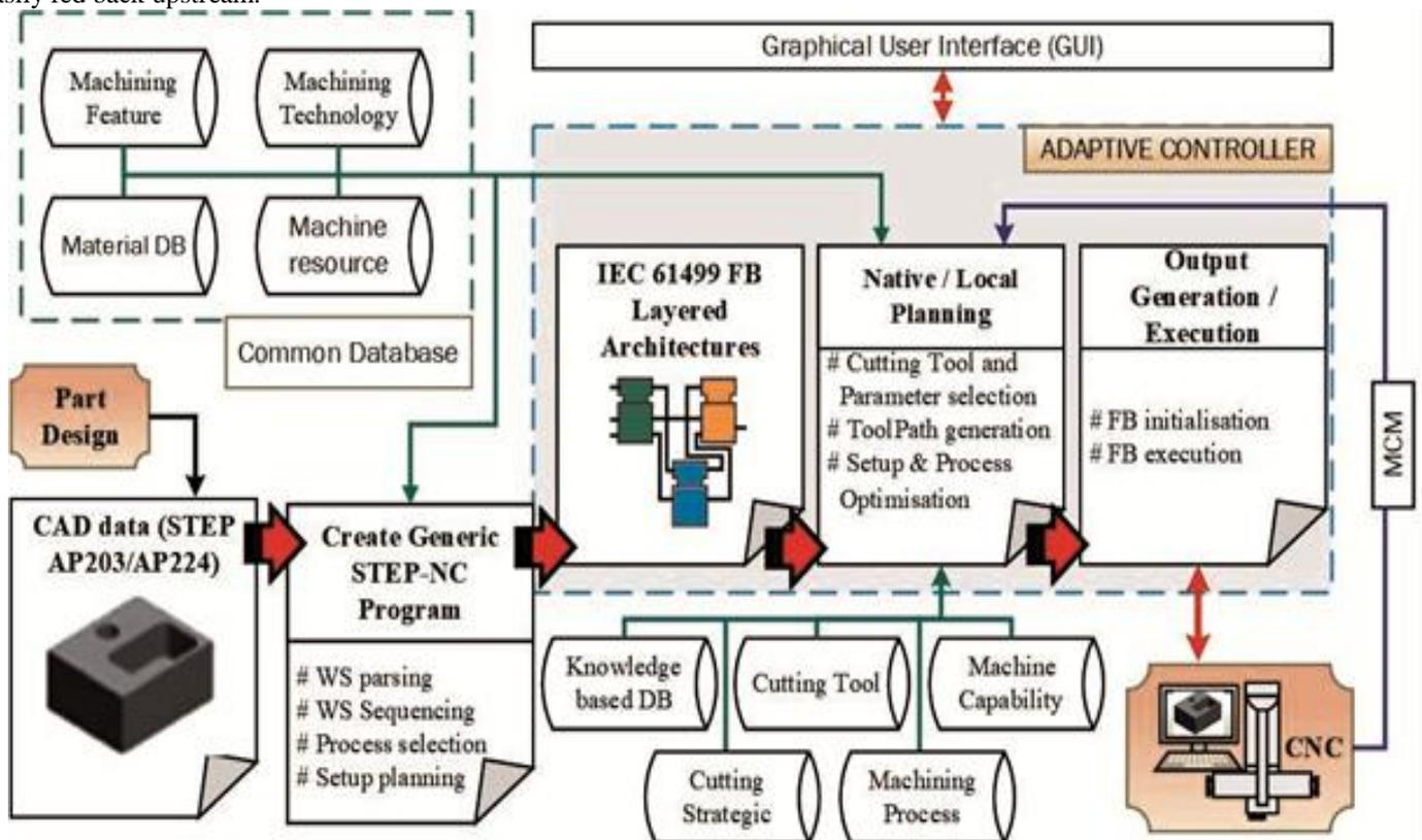
Fig. 2: Proposed Adaptive machining systems
