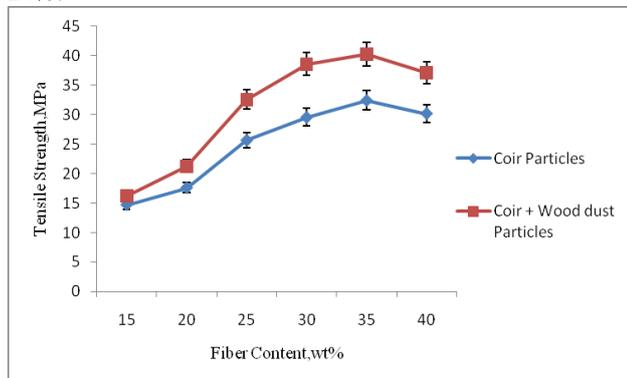
**Fig. 4 Variation of tensile properties of CFRP by the addition of wood dust particles.**
