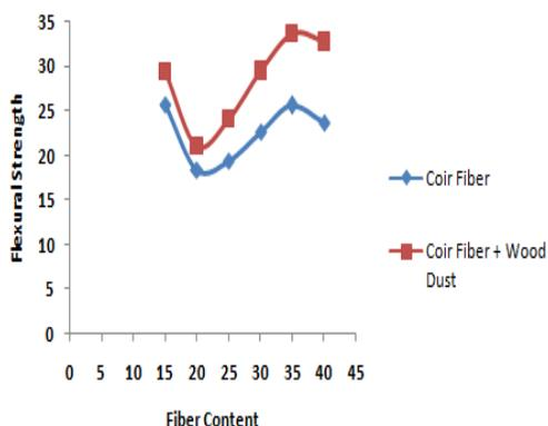
**Fig. 5. Effect of fiber content on flexural strength**
