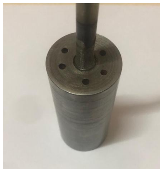
Fig. 4. Displacer linked with the connecting rod
