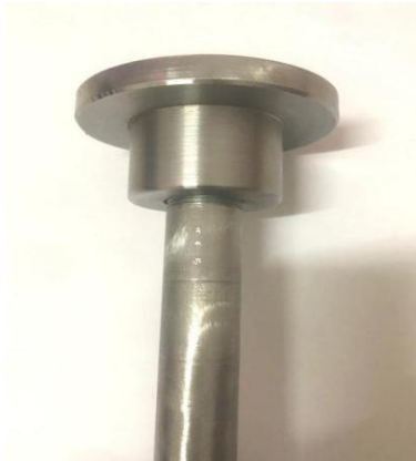
Fig. 5. Power piston linked with connecting rod • Rhombic Drive Mechanism
