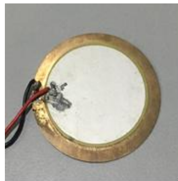
Fig. 4. Round piezoelectric element (diameter = 4.5 cm).
