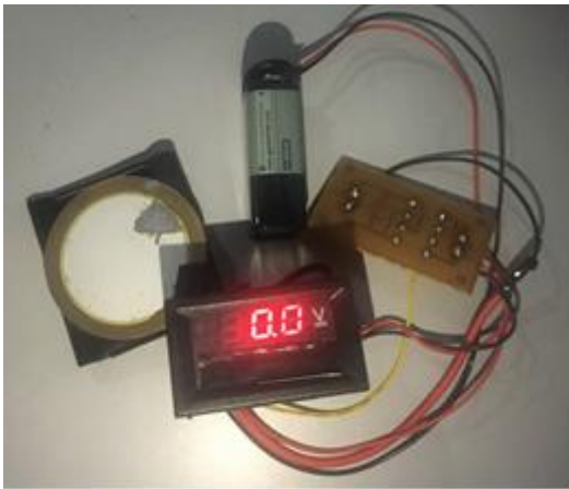
Fig. 8. Overall circuit design with piezoelectric element and digital voltage meter.
