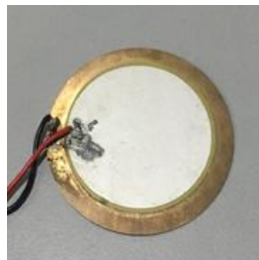
Fig. 4. Round piezoelectric element (diameter = 4.5 cm).
