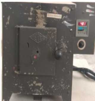
Fig. 3: Muffle Furnace used for sintering process
