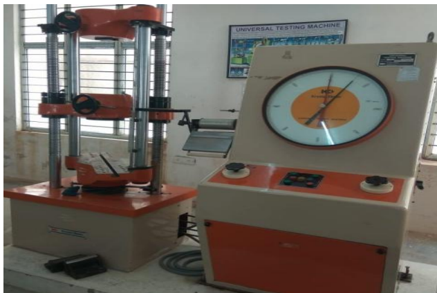
Fig. 2: Universal Testing Machine utilized for compacting process
