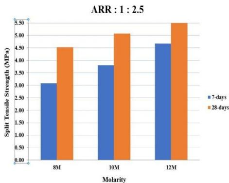
Fig 3.9: Split Tensile strength for varying molarity for AAR 1:2.5
