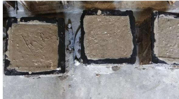
**Fig. 2.2: concrete mould**
