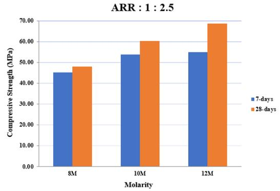
Fig 3.3: Compressive strength for varying molarity for AAR 1:2.5
