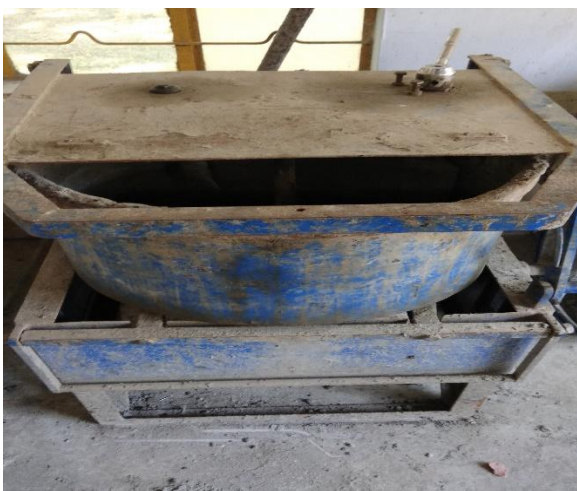
Fig. 1: Concrete mixing machine
