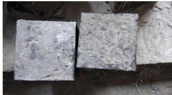
**Fig. 2.3: geopolymer concrete cubes**
