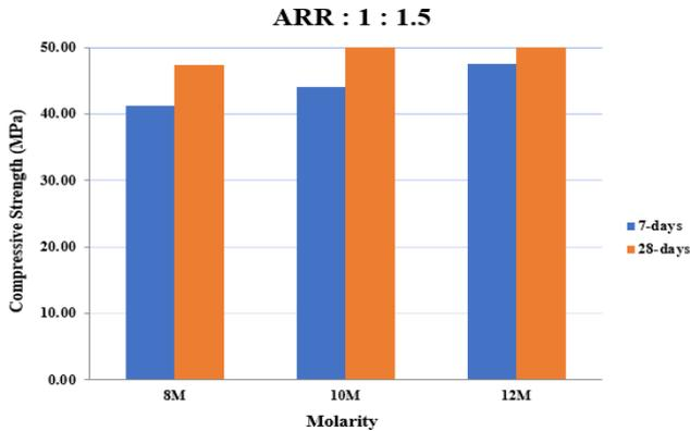
Fig. 3.1: Compressive strength for varying molarity for AAR 1:1.5
