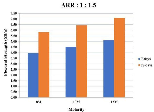
Fig 3.4: Flexural strength for varying molarity for AAR 1:1.5
