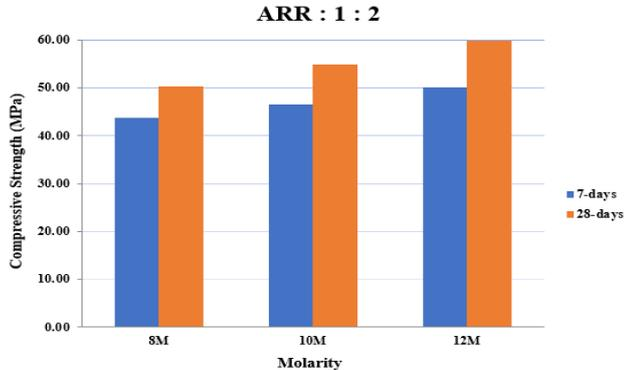
Fig. 3.2: Compressive strength for varying molarity for AAR 1:2
