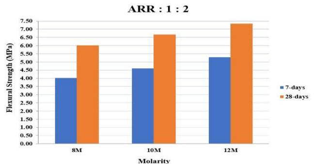
Fig. 3.5: Flexural strength for varying molarity for AAR 1:2
