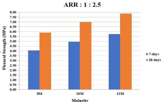
Fig 3.6: Flexural strength for varying molarity for AAR 1:2.5
