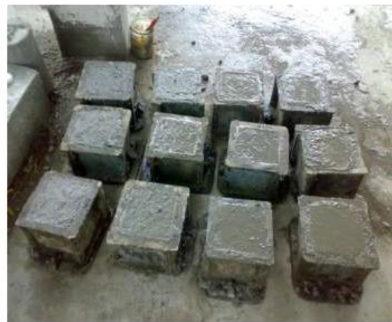
Fig B. Casting of cube specimens
