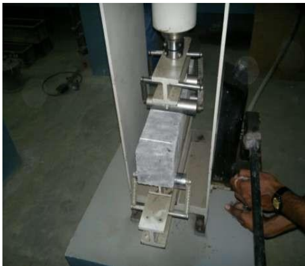
Fig D.2: Test setup for Prism
