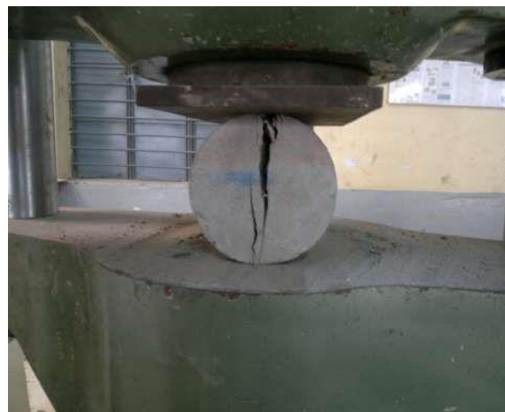
Fig C.1: Split tensile strength test
