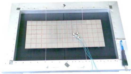
Figure 1. Experimental support for loosely supported steel plate.
