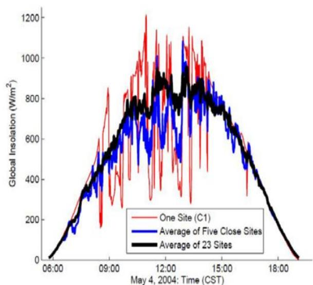
Fig 2: One-Minute worldwide insolation from a single site on a slightly cloudy day, the aggregate of 23sites, and the aggregate of 5 sites that are close to each other
