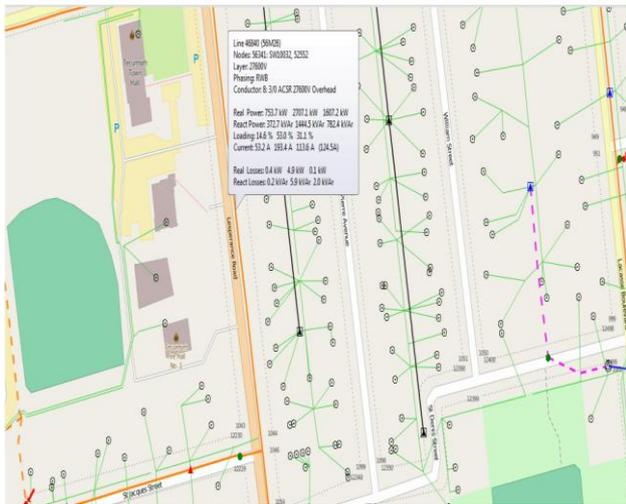
**Fig 5: Analysis of Load Flow on SmartMap**
