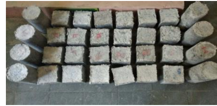
Fig.10. CSRDPFF Cube specimens and CSRDPFF cylinder specimen before testing
