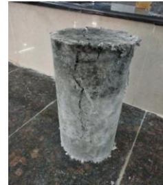
Fig.11. CSRDPFF Cylinder Specimen after testing
