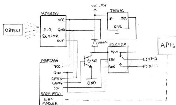
**Figure 4: Circuit diagram of the proposed automated lighting system**
