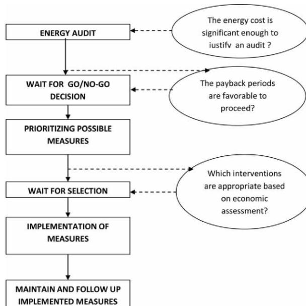
Figure 3: Main phases of an energy management program
