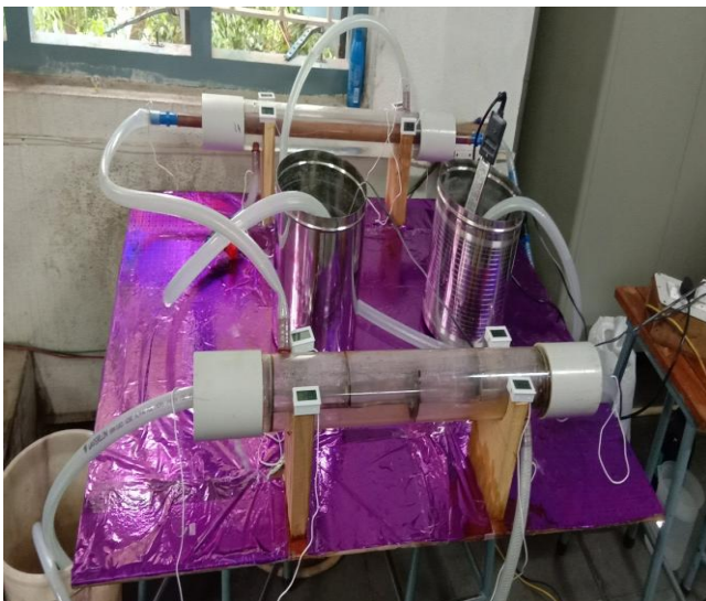
Fig. 1. Combined Heat Exchanger (Tube in tube + Shell and tube) Experimental setup
