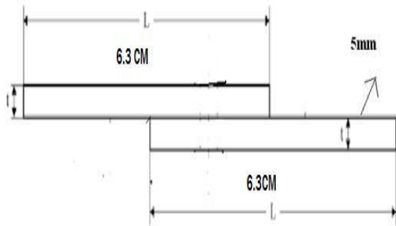
Fig. 10. Flexural strength Lap joint composite specimen
