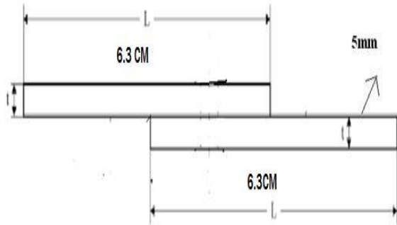
Fig. 10. Flexural strength Lap joint composite specimen
