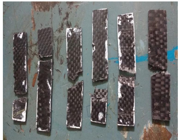
Figure 5.3 Specimens after Impact test.
