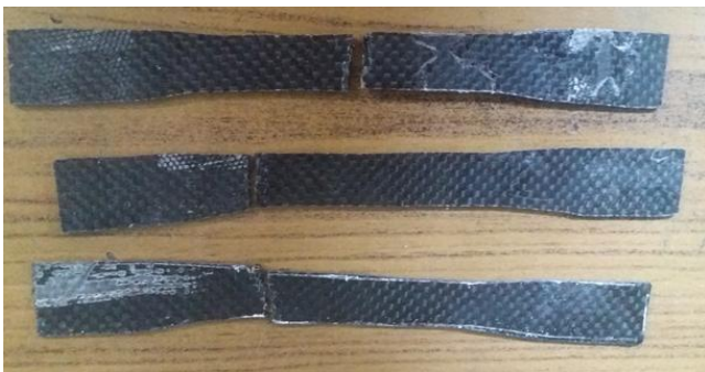
Figure 5.1 Specimen after tensile test.
