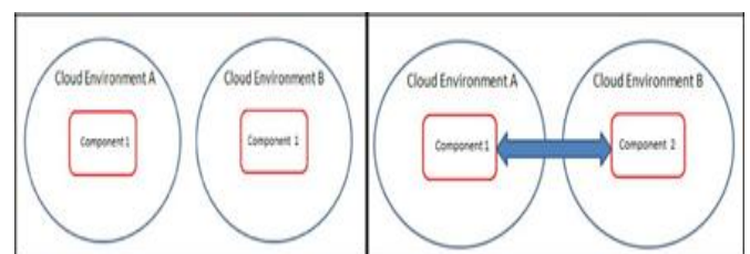
Figure 1: Left: a constituent is transferred from a certain environment to a different one (portability). Right: two constituents of dissimilar environments of the cloud are cooperating (inter-operability).
