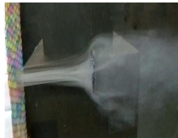
Figure 12: Flow moving around the flat plate
