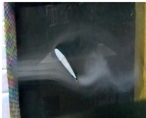
Figure 10(b): Vortex formation at the trailing edge of the airfoil
