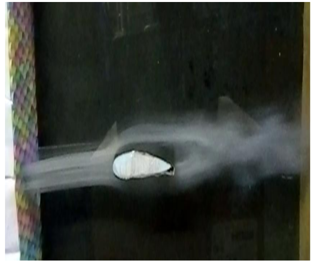
Figure 9 (a): Flow visualization of NACA airfoil 2412
