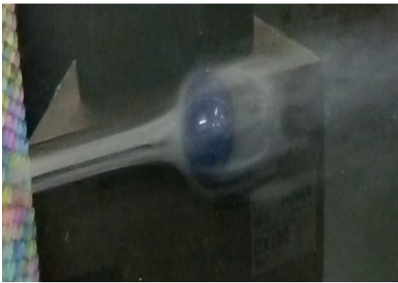
Figure 13(b): Wake and vortex formation at the trailing edge of the sphere
