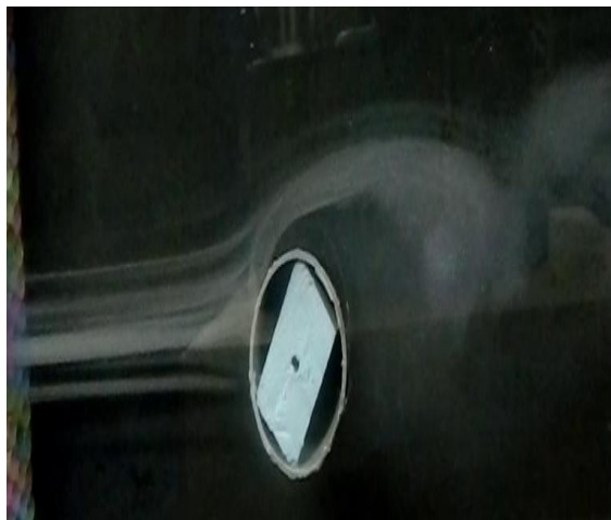
Figure 8 (b): Vortex formation above the cylindrical test object.
