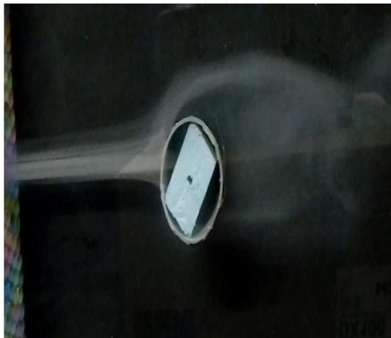
Figure 8 (a): Flow visualization over a cylindrical model
