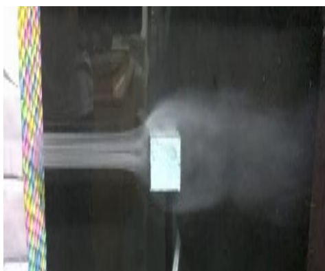
Figure 11(a): Flow visualization over a cuboid model
