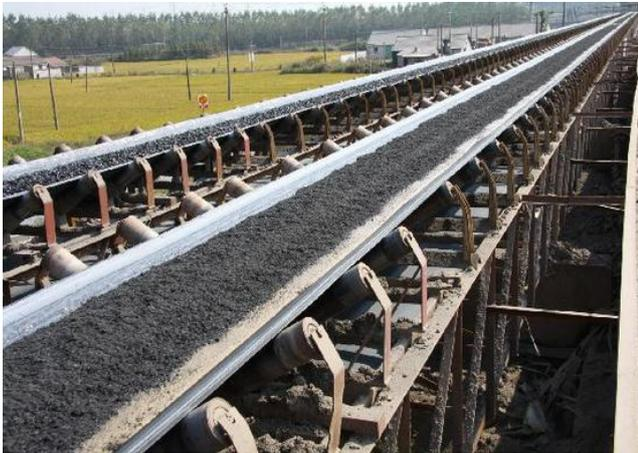
**Fig 4.2:- Conveyor Belt System**
