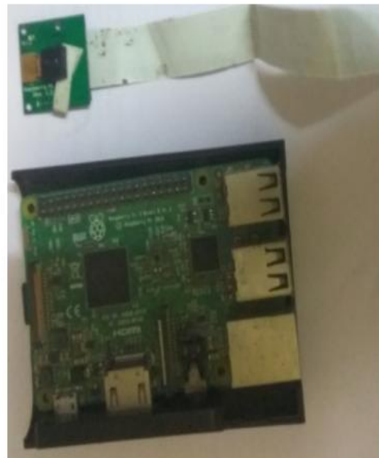
Figure 1: A raspberry pi with the pi camera module
