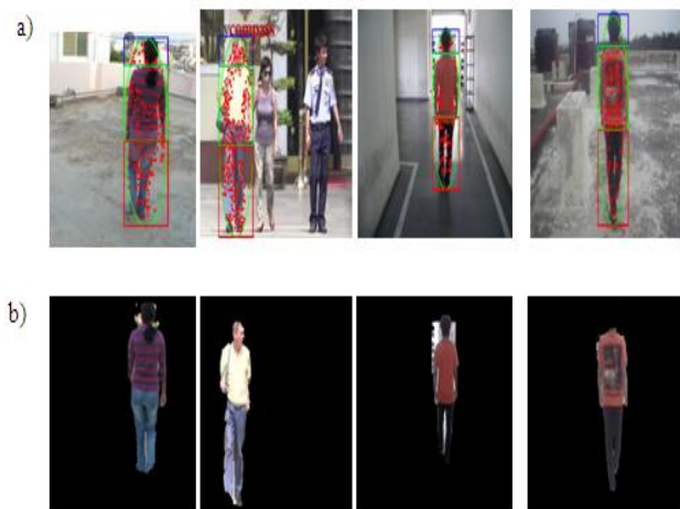
Fig 2: (a) Target manually selected and bounded within ellipse with head, torso, and legs division enclosed in separate boxes. (b) image segmentation results using Grabcut
