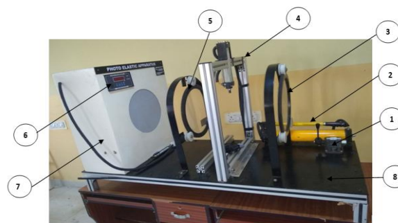
1. One directional valve, 2. Hydraulic pump, 3. Circular polariscope, 4. Mechanical load frame 5. Circular analyzer, 6. Digital load indicator, 7. Monochromatic light source, white light source 8. Leveling table Fig. 3 Experimental setup - Photo elasticity apparatus
