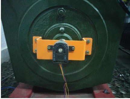
Fig:8 – QEP sensor mounted on DFIG rotor shaft
