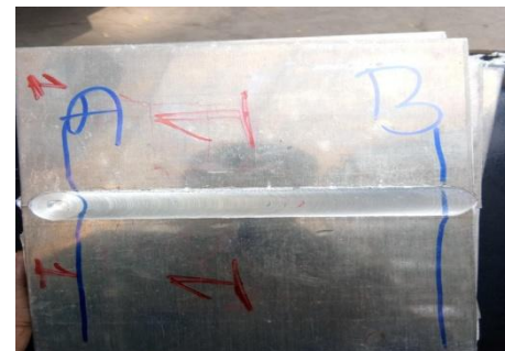
Fig no 5 work pieces after welding
