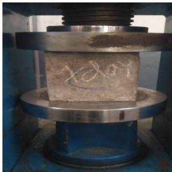
Fig.3: compressive strength of concrete.
