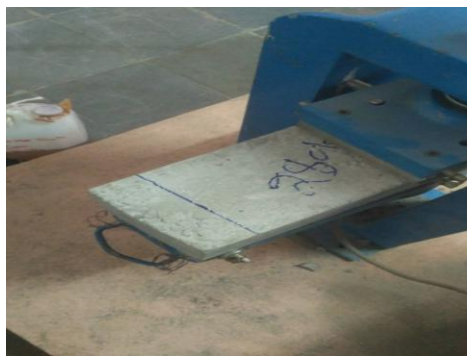
Fig.7: Flexural strength of concrete.
