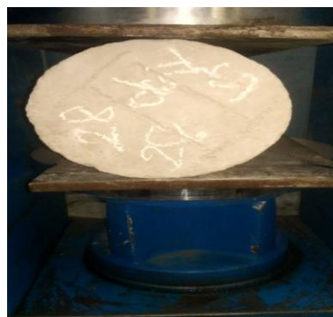
Fig.5: Split tensile strength of concrete.
