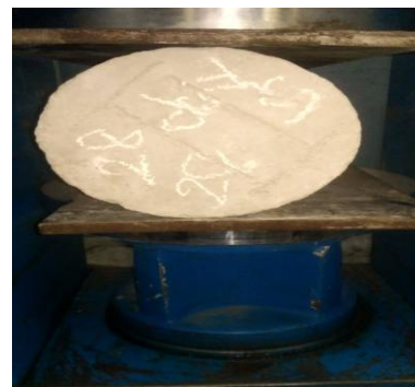
Fig.5: Split tensile strength of concrete.
