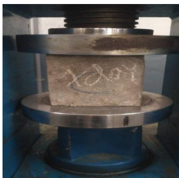
Fig.3: compressive strength of concrete.
