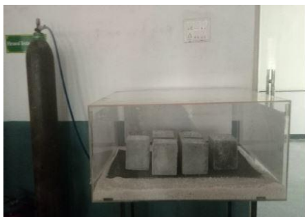
Fig.1: specimens in carbonation chamber
