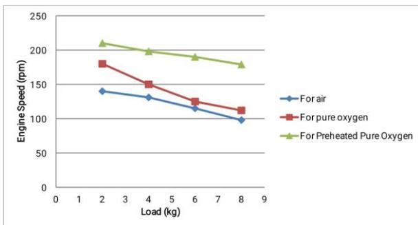
**Fig. 3: Load Vs Engine speed for air and pure oxygen**
