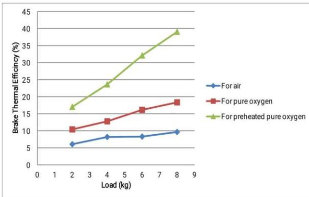
Fig. 7 Graph shows the Brake Thermal Efficiency of the engine for air, pure oxygen and preheated pure oxygen
