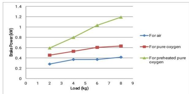
**Fig. 5: Graph shows the relation between BP and Load ( $S_1$ ) for air and pure oxygen**
