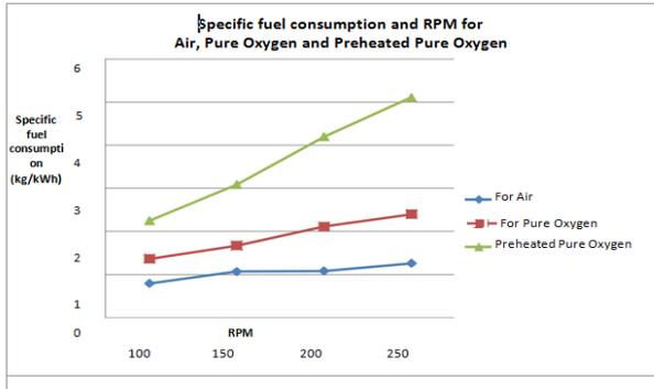
Figure 6 Graph shows the specific fuel consumption of the engine for air, pure oxygen and preheated pure oxygen
