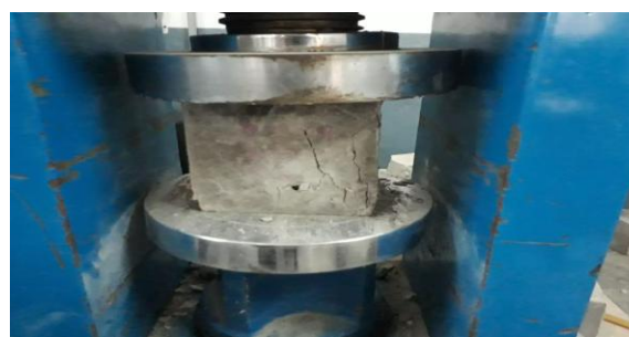
Figure 1:compressive strength test on concrete cubes
