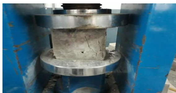
Figure 1:compressive strength test on concrete cubes
