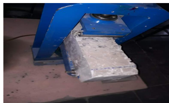
Figure 3: Flexibility Test on concrete beams
