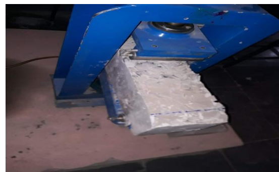
Figure 3: Flexibility Test on concrete beams
