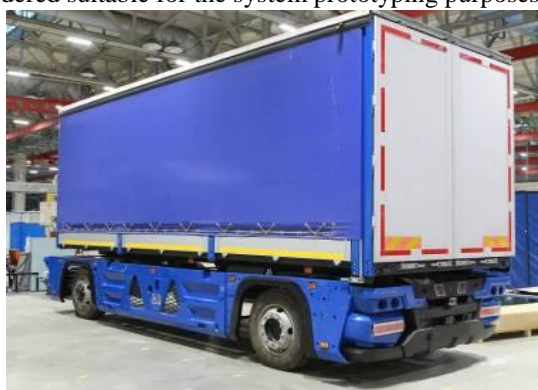
Fig. 3. Special-purpose chassis to be equipped with the automated driving system
