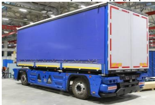
Fig. 3. Special-purpose chassis to be equipped with the automated driving system
