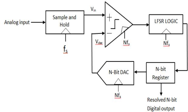
Fig.2. ADC Architecture
