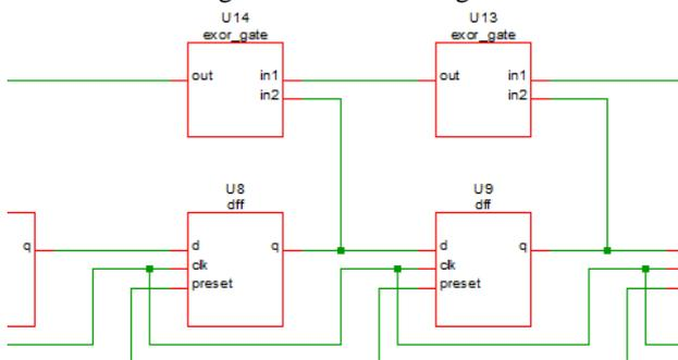
Fig.1. Linear Feedback Shift Register
