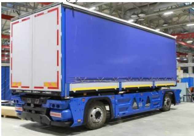
Fig. 2. Modified chassis of a cargo vehicle to be equipped with the automated driving system
