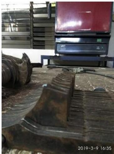
Fig. 1. Preparation of the XU Plastic Shredder blades
