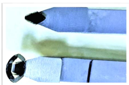
Figure 2.1.1 Single point diamond tool with different nose radius
