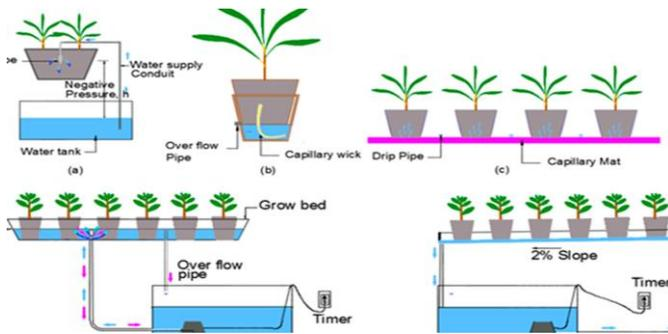
Photo plate 3: Capillary water lift
