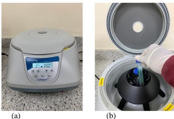
Fig. 3. (a) Centrifuge (b) Sample testing in centrifuge
