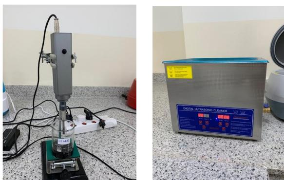
Fig. 4. (a) Ultrasonic Probe (b) Ultrasonic bath
