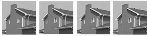
Fig. 5: Comparison of denoising results on noisy image of a house corrupted by WGN of \sigma=25 . (a) NLSM (PSNR of 33.14), (b) BM3D (PSNR of 32.89), (c) PLOW (PSNR of 32.70) and (d) proposed OPSS (PSNR 34.34).
