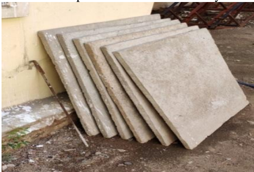
Fig.1 Ferro-Geopolymer slabs kept for curing
