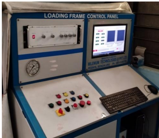
Fig.4 Loading Frame Control Panel
