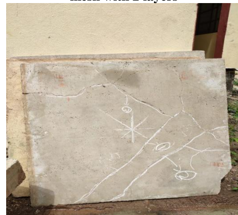
Fig. 7 Ferro-Geopolymer square welded mesh with 2 layers
