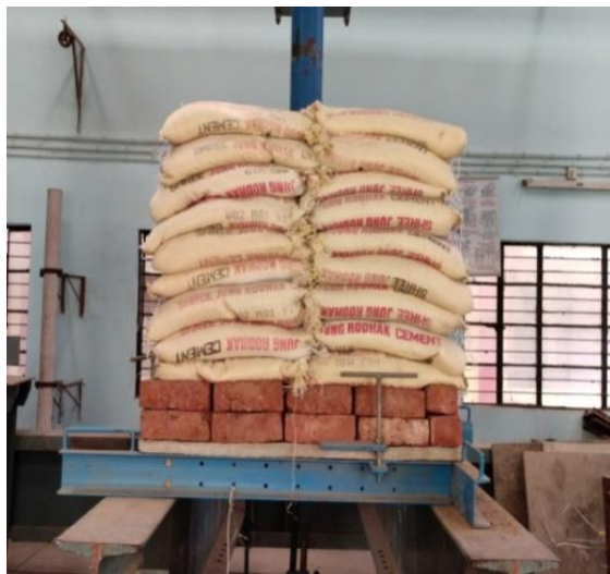
Fig.5 Layer wise load applied on slab
