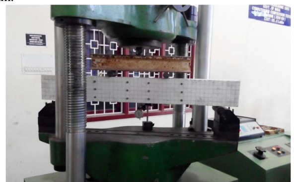
Fig. Beam test set-up
