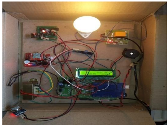
Fig 2: Prototype Coal miners safety monitoring system execution
