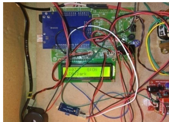
Fig 3: LCD displaying temperature, gas, LDR values
