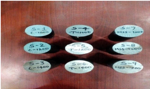
Fig 2. Work pieces before machining (EN19 steel)
