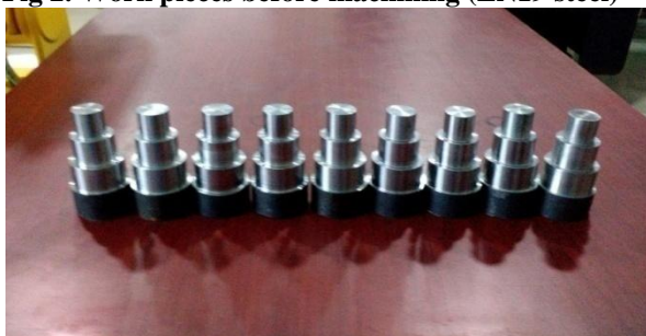
Fig 3. Work pieces after machining (EN19 Steel)
