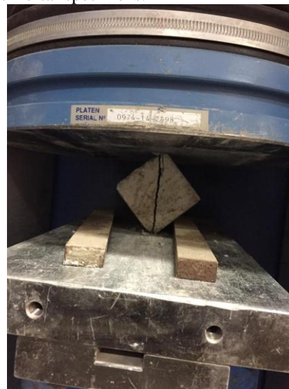
Figure 4: Splitting Tensile Test Setup
