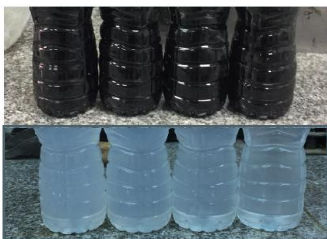
Figure 3: CNT and NCL solutions after sonication and directly prior to adding to the cement paste
