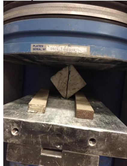
Figure 4: Splitting Tensile Test Setup
